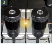
Join the end wire from drum 1 with the start wire from drum 2 using the Butt Welder.
