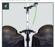
When wire from drum 1 runs out, the transfer arm will switch over to drum 2. Simply replace empty drum and repeat steps 1 – 3.
